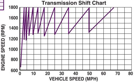
T-310ME w/1800 RPM ENGINE, REAR RATIO 4.42 AND 11R22.5 TIRES (BASED ON 498 TIRE REVS PER MILE)
