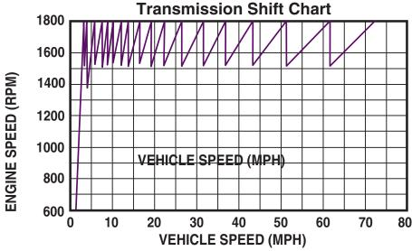
T-31821 w/1800 RPM ENGINE, REAR RATIO 4.17 AND 11R22.5 TIRES (BASED ON 504 TIRE REVS PER MILE)
